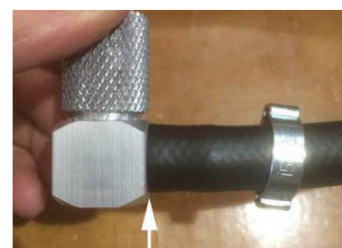
4. Fit hose over hose coupling get hose contact the coupling wall.
